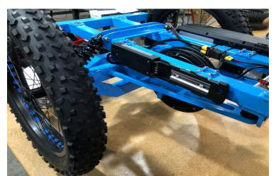
Installing the battery is quick and easy. First, locate the battery sled that is already mounted onto The Rig. In most cases you'll find it on the side of the frame behind the seat, In the picture on the left, you can see the battery sled mounted to the RIG.
