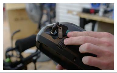
If the battery remains securely in place when after pulling upwards, locate the key hole and insert your key. Turn your key clockwise (to the right or toward the back of the battery) to engage the locking pin. Try to slide the battery out of the sled. If it stays in place, you have successfully engaged the locking pin and your battery is secure. You may stow away your key in a safe place and continue to the next section "Console Operation".
