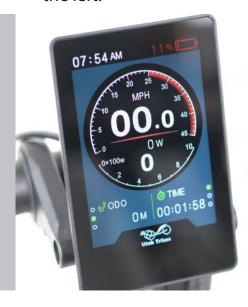
Your console shows you a number of different settings. The top left corner of the screen displays the time. The top right corner of the screen displays your remaining battery (this can be set to percentage or voltage in the settings). In the center of the console is your speedometer and MPH readout. Your console also displays the wattage draw from your motor.
