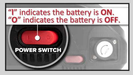
Once your battery is in the "I" or "ON" position, find the power indicator on top of the battery. This indicator has four (4) LED lights that are meant to show your battery's power level. While pressing on the power button, the LED lights will light up.
