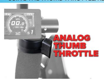
Our UTCustom Hub Motor system include a thumb throttle. This is usually located on the left handlebar near your console. It is an analog throttle, meaning the more you more you push it forward, the more power your motor will put out.
