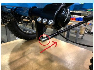
For easy side access to The Rig's seat, drop down the steering handles by sliding the silver coupling forward at the base of the steering handle. Pushing arm cupling forward will allow the coupling to release from the joint. You can then lay the steering handle down out of the way. After transfering into The Rig pull up the arm so it is parallel with the other steering handle and reattach the joint in the same fashion. It is helpful to have a friend or assistant to help with this part.
