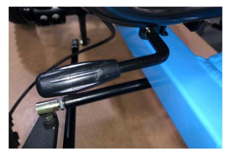
To slide the seat forward or backwards, pull up on the lever under the right side of the seat. While lifting the lever, slide the seat forward or back to fit your desired position.
