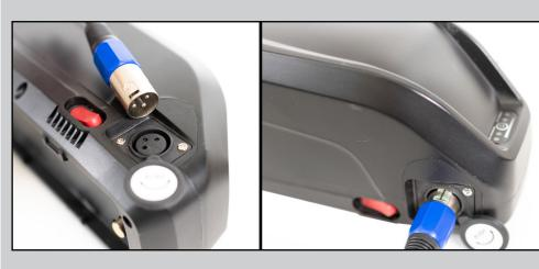
Be sure to line up the three prongs of the charging plug with the three corresponding holes of the charging port.
