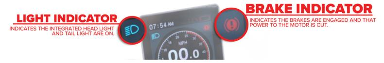
If you have an integrated headlight/ tail light, you can press and hold the plus (+) button to turn on your lights. The light indicator will then be displayed on your screen in the top left-hand corner. To turn your lights off, press and hold the plus (+) button again.
